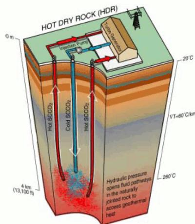
Figure 2 Enhanced geothermal system using supercritical CO<sub>2</sub>. Source Donald Brown, LANL.
