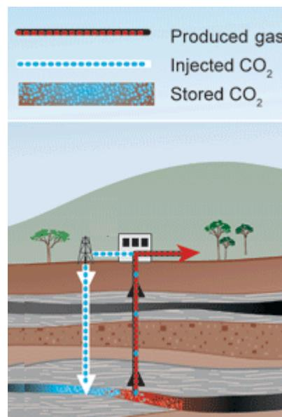
Figure 3 Enhanced coal bed methane recovery. Source LBNL
