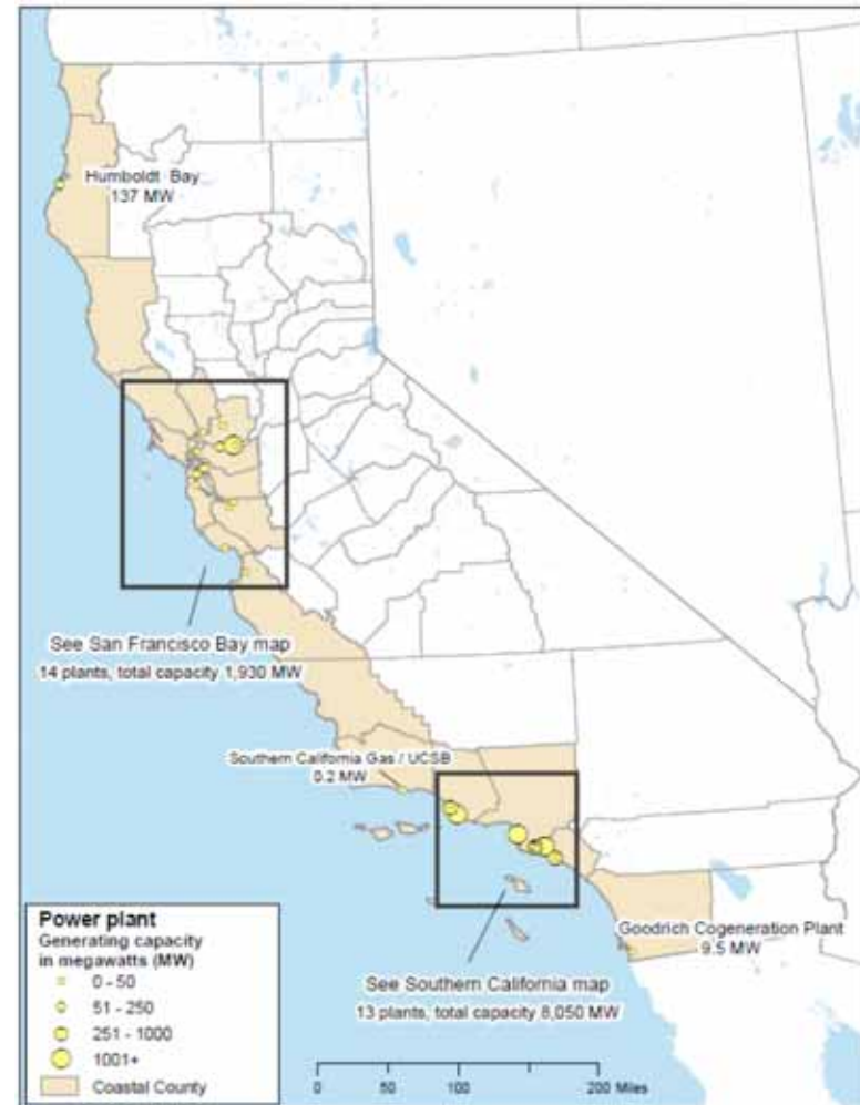
Power plants vulnerable to a 100-year coastal flood with a 1.4 meter sea-level rise
